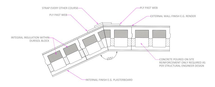
DURISOL BLOCKS CUT ON SITE TO REQUIRED ANGLE. BLOCK CUT TO ALLOW FOR FULL WIDTH OF INSULATION AT CORNER. IF SNUG FIT CANNOT BE ACHIEVED BETWEEN CUT BLOCKS UTILISE TEMPORARY SHUTTERING TO CONCRETE POUR
