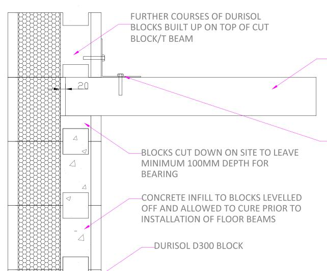
PCC FLOOR PLANKS OR BEAM AND BLOCK FLOOR AS SUPPLIED AND SPECIFIED BY OTHERS
