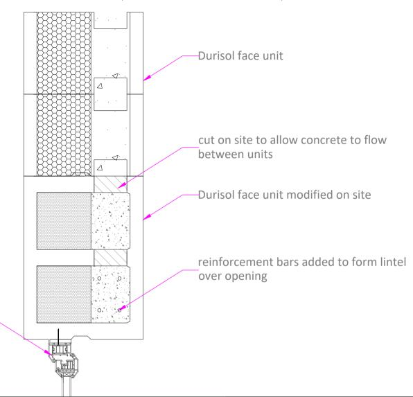
window unit fixed with screw through frame into block or with proprietary strap fixed to internal reveal. gap between window and durisol reveal filled with a suitable sealant.
